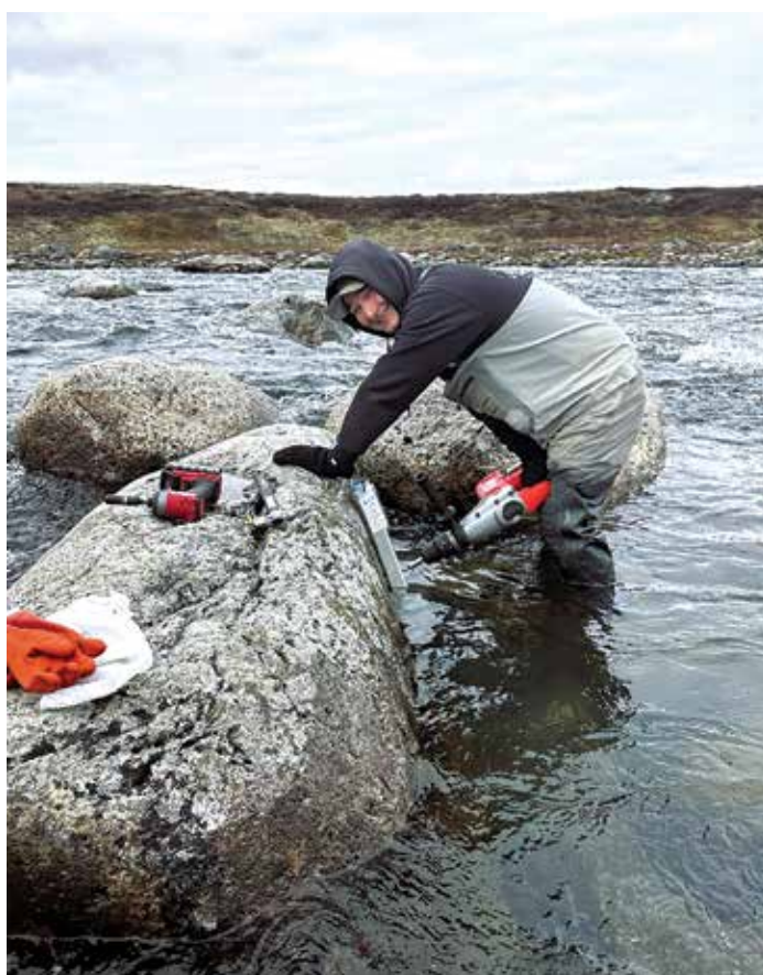
Near Aupaluk this fall, Paulusie Papak, NRC Wildlife technician, anchored a logger to a boulder in Allavik River (left) to measure the amount of water flowing in Qingaujaq River (right).
