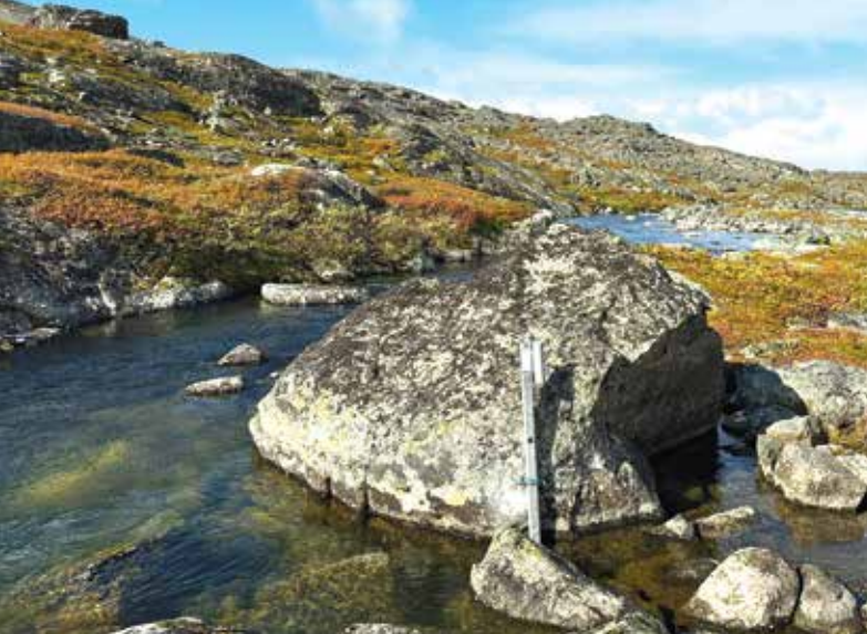
Water level and temperature recorder installed in Kuukallak River near Inukjuak during fall 2025 fieldwork.
