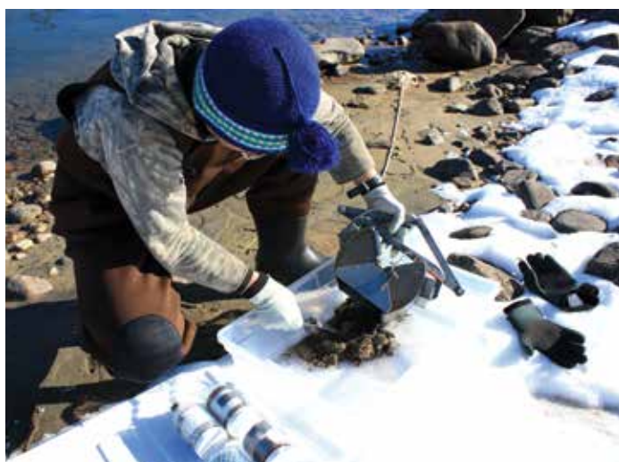
Fieldwork at the Vachon River west of Kangirsuk, summer 2013. Collecting sediment samples for contaminant analysis.
